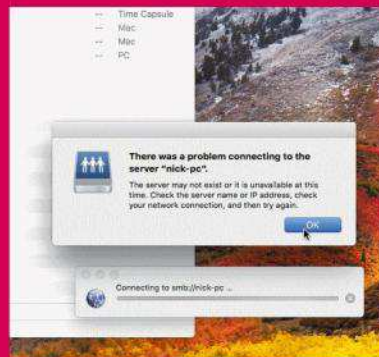
If your Mac cannot connect to one PC but others work fine, the problem lies with that specific PC.
